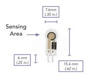
The FlexiForce A101 is our smallest standard piezoresistive force sensor. The A101 design is optimized for high volume manufacturing and is ideal for embedding into products and applications. This sensor is available in low and high quantities off-the-shelf, ideal for an easy proof of concept. The A101 sensor is designed to use with your own electronics or multimeter.
